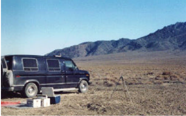
First use of the WR-4B van-based VLF receiver with roof-top whip antenna assembly in Black Rock Desert of north-western Nevada, 11 October 1992. Later, after losing this antenna assembly in Oregon, the more successful rear-door mounted vertical was developed for the Big Canadian trip of September 1993.
